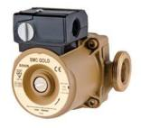
The pumps are of a drum motor design using hard coated shaft and bearings supporting a moulded impeller and rotor. Motor cooling and bearing lubrication is carried out by the pumped water. Models offer a single or variable speed
